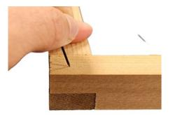
To secure each bar, apply wood glue to all touching surfaces and fasten with a gimp pin. Before the glue sets, measure both diagonals from corner to corner. If the diagonal measurements are unequal, adjust the frame by pushing or pulling on the corners until both measurements are the same, which will make the eke square.
